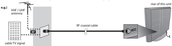
\* Once connections are completed, turn on the unit and begin initial setup. Channel scanning is necessary for the unit to memorize all available channels in your area. Refer to "Initial Setup" on page 17.
